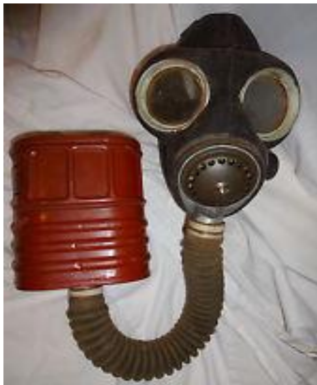
WWII British Military mask. The filters contain crocidolite asbestos. Masks, filters and carrying bags can be contaminated
